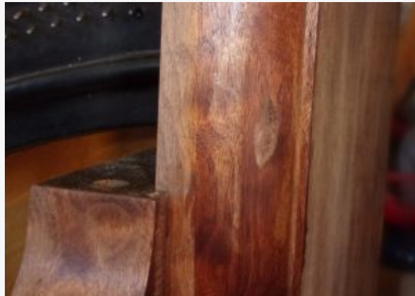
The patch glued and sanded level
