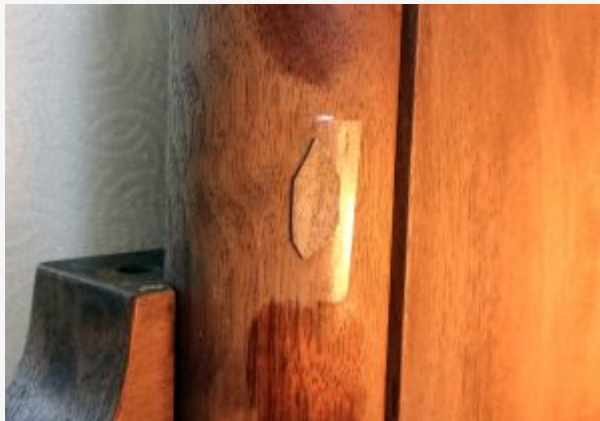
Laying out the patch
