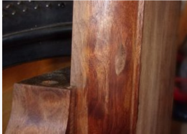
The patch glued and sanded level
