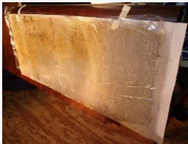
An example of soaking an old shell finish with alcohol for removal
