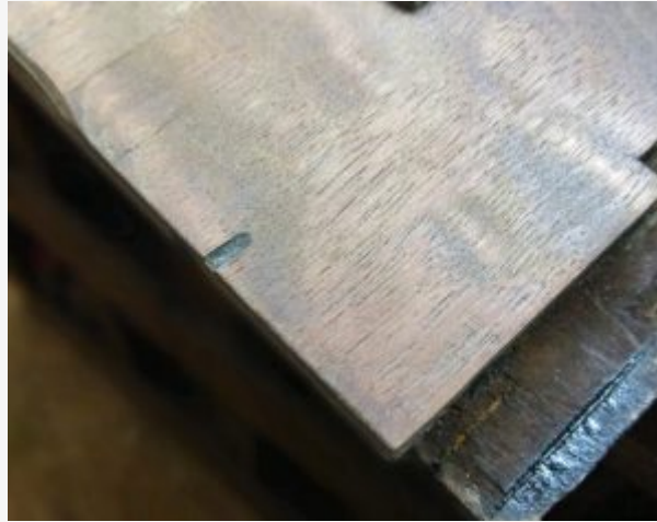
A small veneer chip-out
