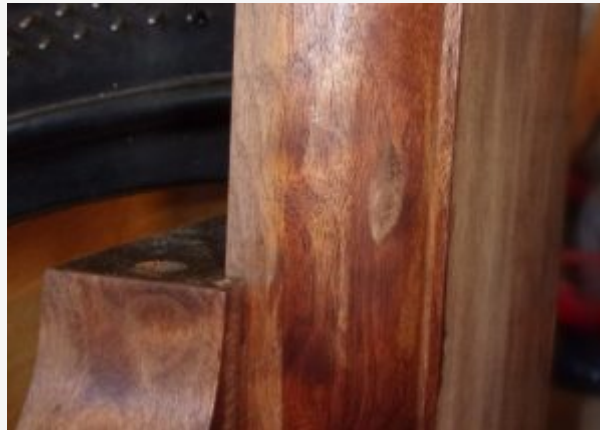
The patch glued and sanded level
