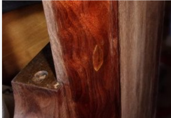
The patch after staining
