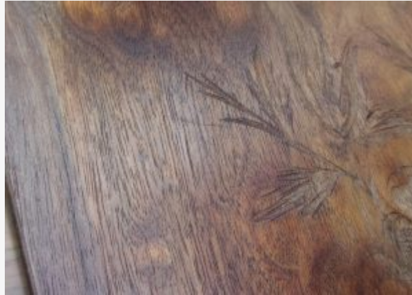
A scratch that looks to be a good candidate for a steam repair
